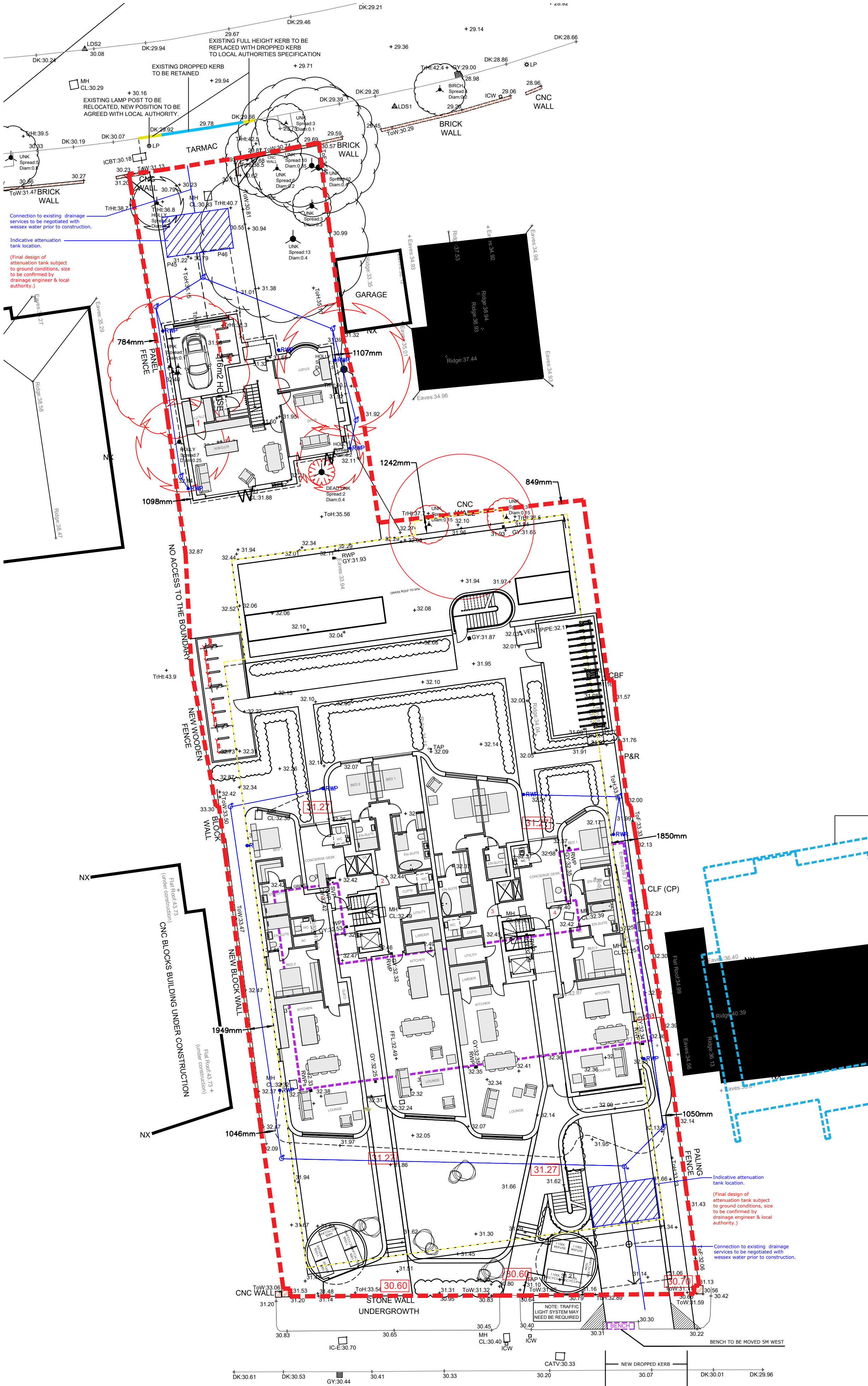
INDICATIVE DRAINAGE PLAN: BASED ON TOPOGRAPHICAL SURVEY INFORMATION SCALE: 1:200
